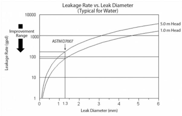
ASTM D7007 specifies a 1.3mm (0.05in.) test leak. The equipment and survey parameters are set up to detect leaks this size under near worst-case conditions.
