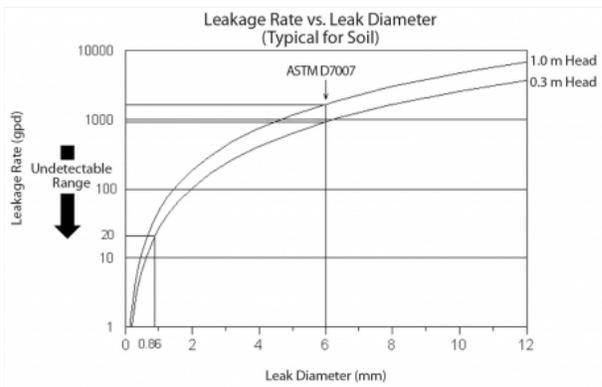
ASTM D7007 currently specifies a 6mm (0.236in.) test leak. Again, as part of the leak-location procedure, equipment and survey parameters are set up to detect leaks this size under near worst-case conditions. This diameter and the corresponding leakage rates for water heads of 0.3m (1ft) and 1.0m (3.3ft) are also shown in the figure.
