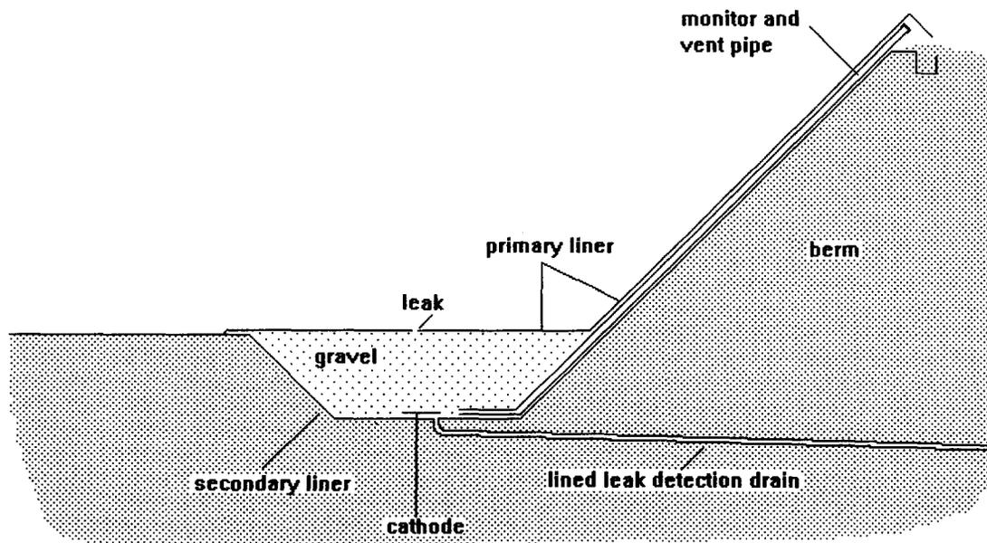
FIG. 6. Cross Section of Leak Detection Sump
