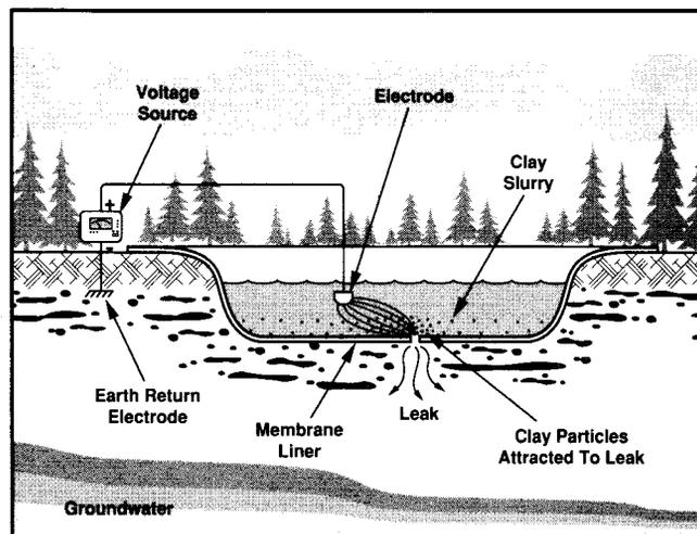
FIG. 1. Principles of Electrophoretic Leak Sealing Method
